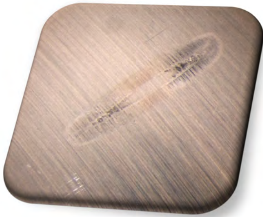
Figure 15 Representative standstill mark after a 6-hour test with a TMP ester oil
