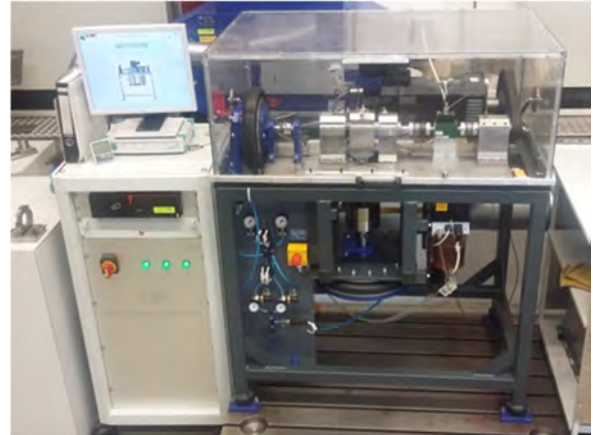
Figure 0-6: Overall View of the Bearing Friction Test Rig and control system.
