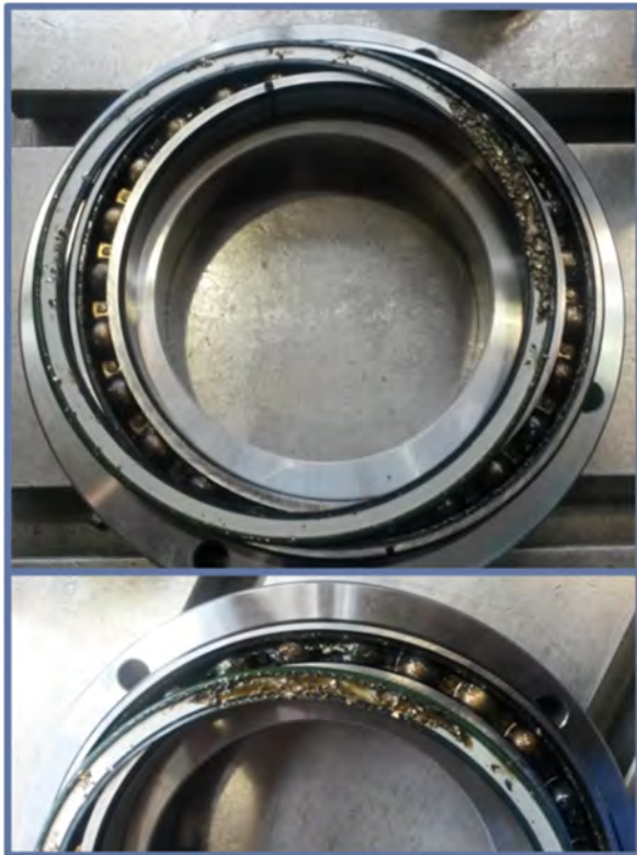
Figure 1-2: Hot-running of a test rig bearing.
