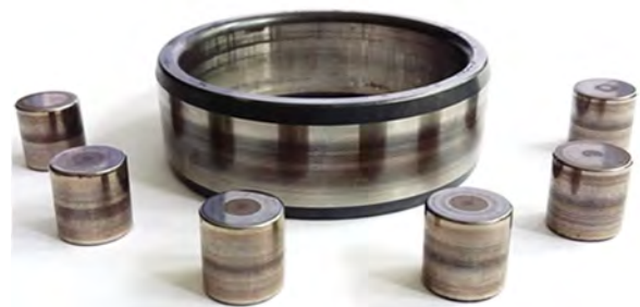
Figure 0-33: Cleaned inner ring and selected rollers of the test bearing after a long run under oscillations.
