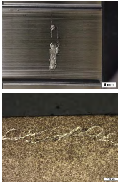
Figure 3-3: Macroscopic damages on IR (top). Subsurface WECs (depth of 100 – 360 \mu\text{m} ) without pitting on raceway (bottom)
