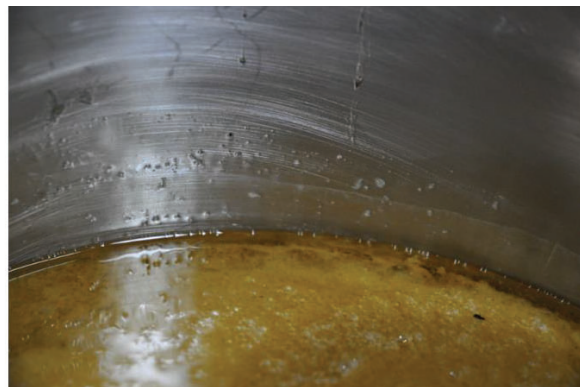
Figure 14: Noticeable oil residue in the dirt water reservoir – 15,000 km friction distance, 5 h / 10 s exposure
