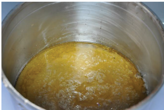
Figure 14: Noticeable oil residue in the dirt water reservoir – 15,000 km friction distance, 5 h / 10 s exposure
