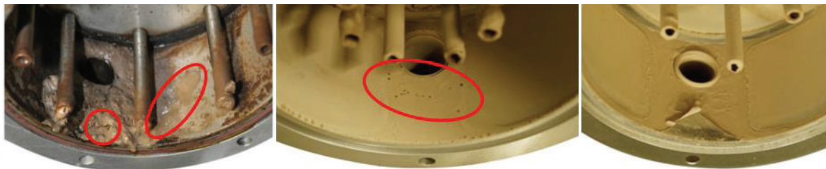
Figure 17: Oil residue in the test cell – 15,000 km, exposure 5 h / 10 s (left: extensive leakage – centre: flung-off oil drops – right: no leakage)
