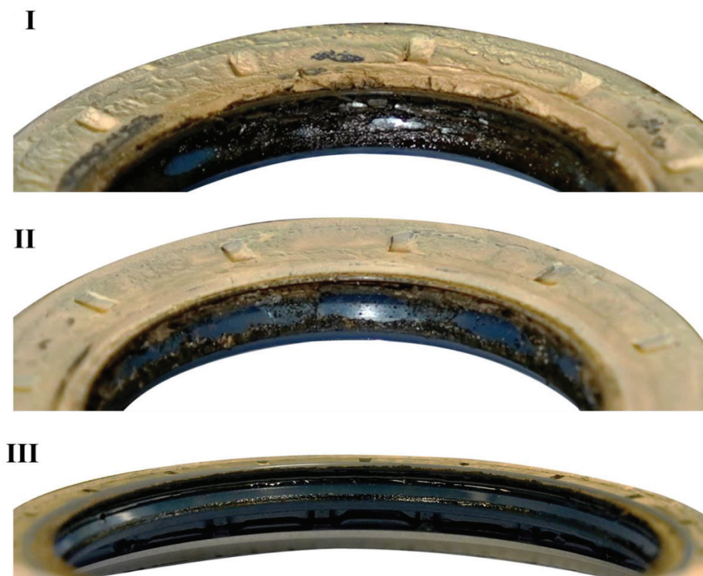
Figure 15: Grease evaluation at the pressed-in RSS
